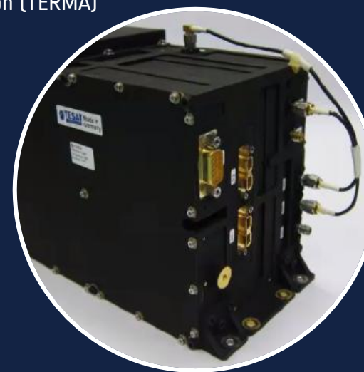
Miniature Active Pixel Sensor based Star Tracker to support PLATO mission (TERMA)
