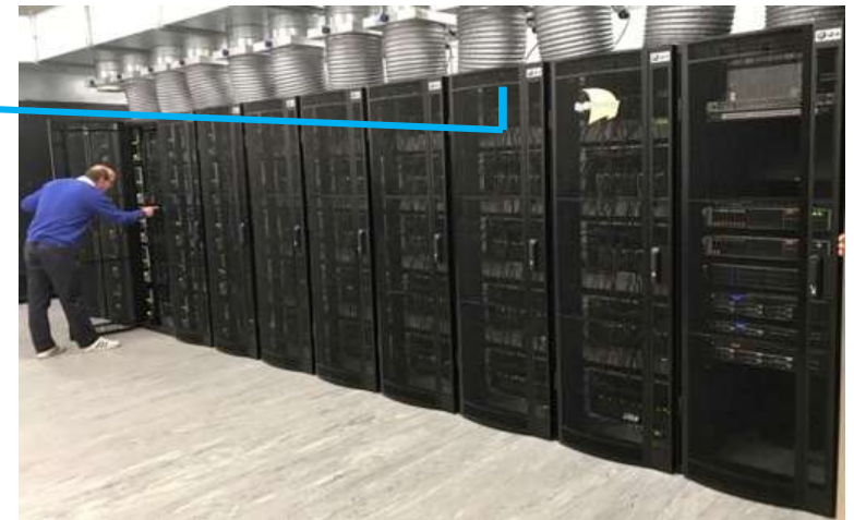
SpiNNaker racks (1M ARM cores)
